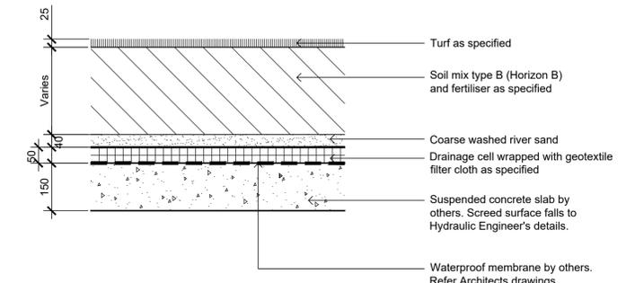
**Detail Turf on Suspended Structure**
